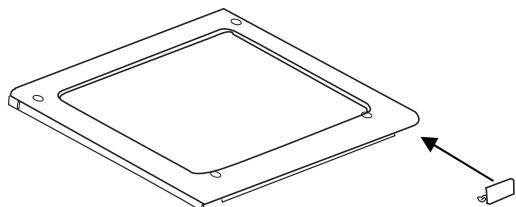
5. Remove the upper hinge pin, transfer it to the left side and tighten securely, then put the hinge bracket in a safe place.
