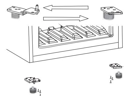
8. Replace the lid by fitting the upper hinge pin into the hole in the upper door, securing it with the 4 screws. Refit the screw covers.
