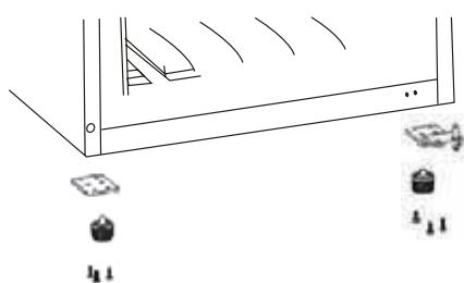
7. Unscrew and remove the bottom hinge pin, turn the bracket over and refit the pin. Refit the bracket with the bottom hinge pin.
