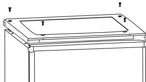
3. Use a flat-bladed screw driver to remove the top cover plate from the front.
