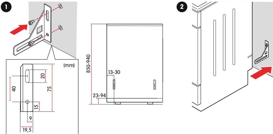
1. Fasten the bracket to the wall using the supplied screws and anchors.
