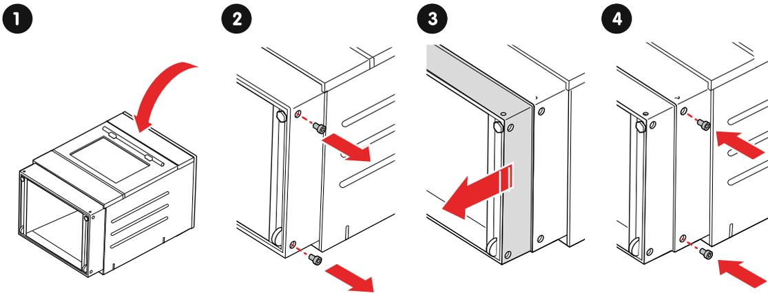
1. Lay the cooker down on the floor on its back.
