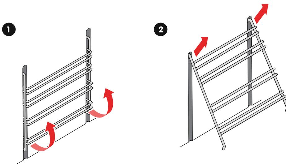
1. Pull the bottom side of the guides out from the oven wall.
