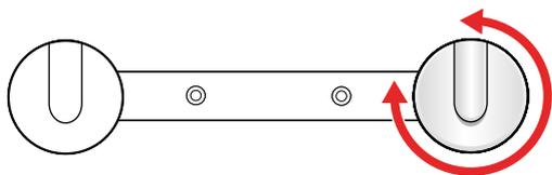
1. Turn the temperature selector clockwise to increase the temperature or anticlockwise to lower the temperature.
