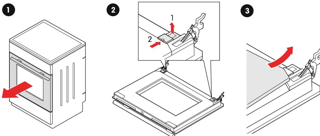
1. Remove the oven door from the appliance (section "Replace the oven door", [page 20](#)).
