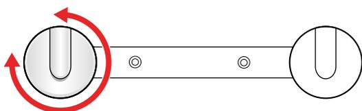
1. Turn the cooking mode selector clockwise or anticlockwise to switch between the available modes.
