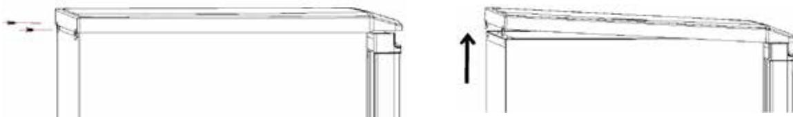
4. Unscrew the screws from the top hinge and remove the hinge.
