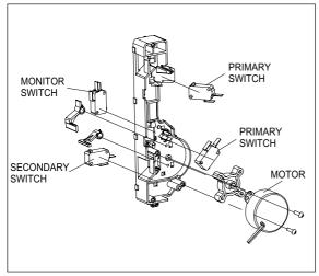
Fig.2 For Electric Door Control Built-In Model
