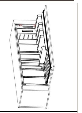
4) The door of the cabinet is opened to the maximum angle, and the door of the refrigerator is opened to the corresponding position. Sliding the block to make inner edge align with the door edge, then fix the block to the door with screw and flip the edge of the slider to cover the screw cap.
