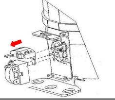
8) Loosen the screw of the compressor bottom plate, remove the floor together with the compressor from the box.
