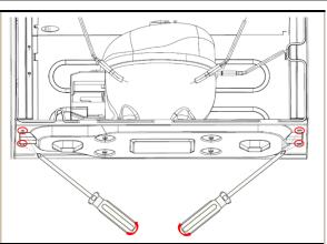
9) Use the wrench to remove the bolts by steps 4567, replace the compressor and reverse process can complete installation.
