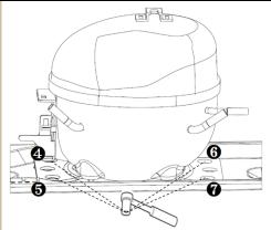
10) Use Pipe cutter cut off the condenser tube **8**, then Shear off capillary **9** by the capillary tube scissors.
