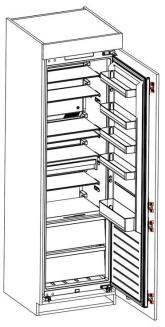
5) The sealing strip in the accessory is sealed in the gap between the cabinet and the refrigerator.
