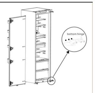
4. Exchange the upper hinge and bottom hinge, then assemble them.
