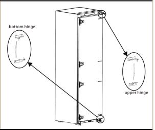
5. Assemble the hole caps, remove the fixed block of fridge door and rotate it for 180°, assemble it on the other side of the refrigerator door.
