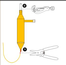
11) Replace the compressor and welding the compressor pipeline. • Welding the low-pressure muffler. • Welding the process pipeline. • Welding the high-pressure exhaust pipe.
