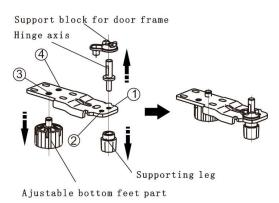
8. Set the door into its new place making sure the pin enters the bushing at the lower frame section.
