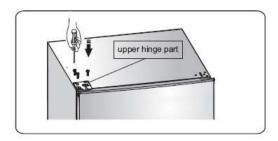
10. Put the screw hole cover and upper hinge cover (left) as follow diagram.
