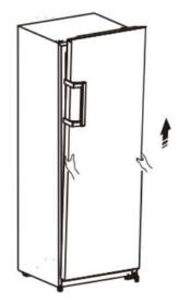
5. Loose screw ② and screws ⑤ , detach part ① and part ③ part ④ . Replace part ① to the right side and tighten securely with screw ② . Replace part ③ and part ④ to the left side and tighten securely with screws ⑤ .
